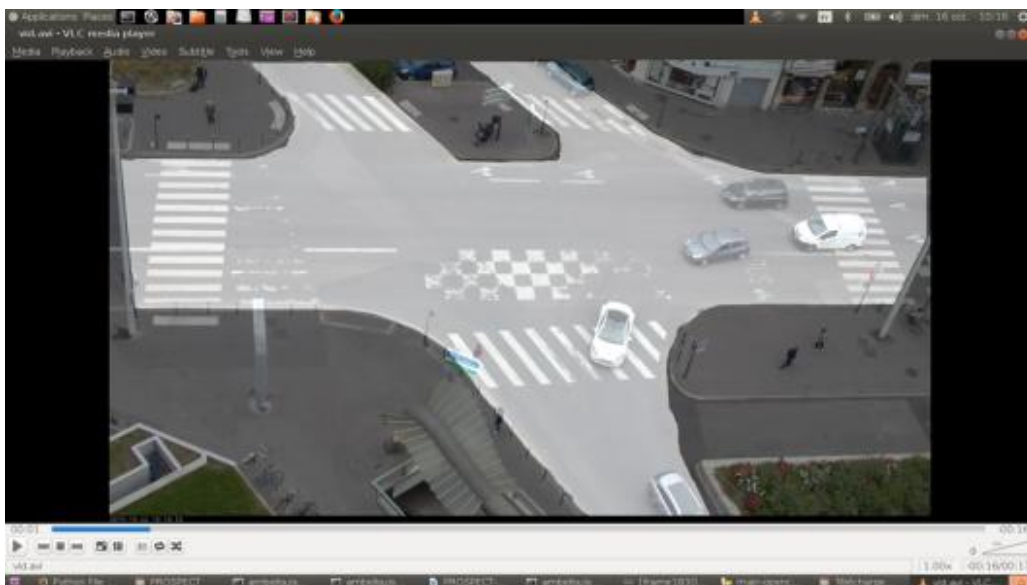
Figure 8: Mask applied to exclude non relevant areas of the scene
