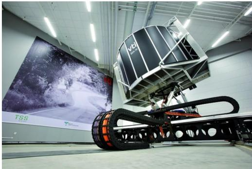
Fig. 16 The Sim IV, moving-base driving simulator located at the VTI site in Gothenburg, Sweden.
