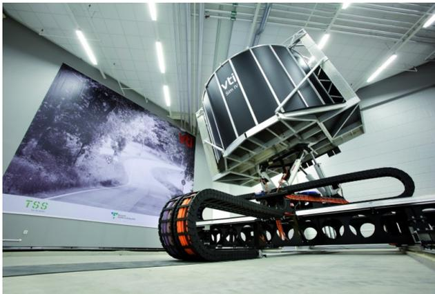
Figure 3.7: The “Sim IV” driving simulator used in Paper V.
