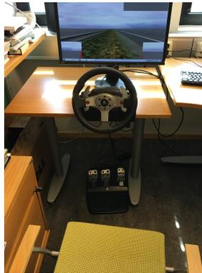
Figure 3.5: The desktop driving simulator setup.
