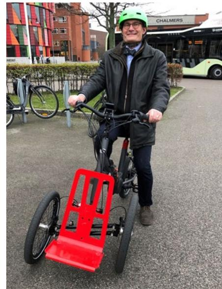
*Figure 17: In collaboration with Cycleurope SAFER is conducting a project to develop a new type of safer three-wheel bike. As it has just three wheels, it becomes more stable.*
