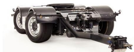
Figure 5: Revere's active dolly is now considered as a full-scale research platform for long vehicle combinations.
