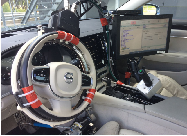
Fig. 9: Steering robot used for executing driving trajectories.
