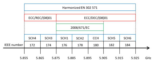
Figure 2: ITS frequency band in Europe with corresponding channel names and IEEE channel numbering
