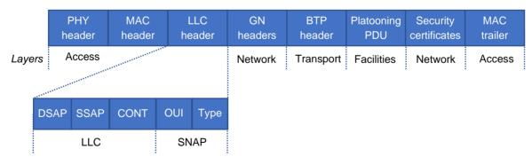
Figure 6: LLC encapsulation of the platooning PDU
