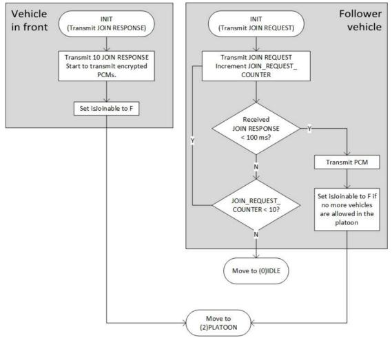
Figure 11: JOIN procedure
