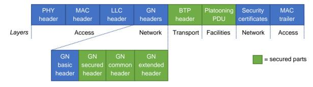
Figure 5: Secured GN encapsulation of the platooning PDU and BTP header
