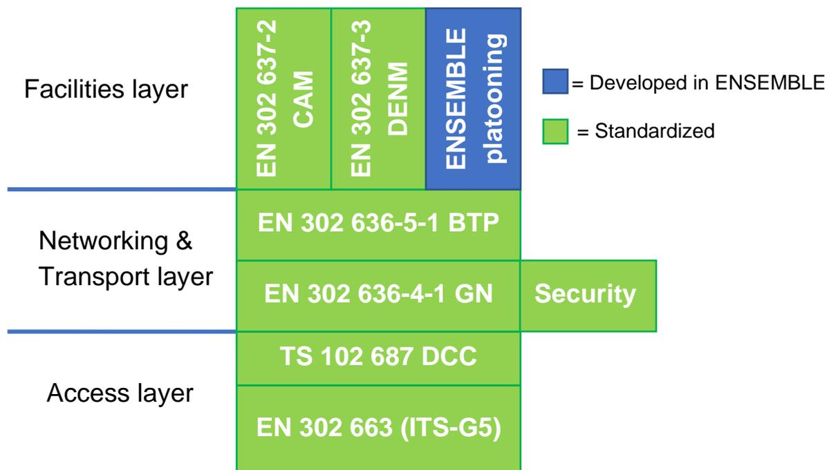
Figure 1: C-ITS protocol stack with standardized protocols and the ENSEMBLE platooning protocol
