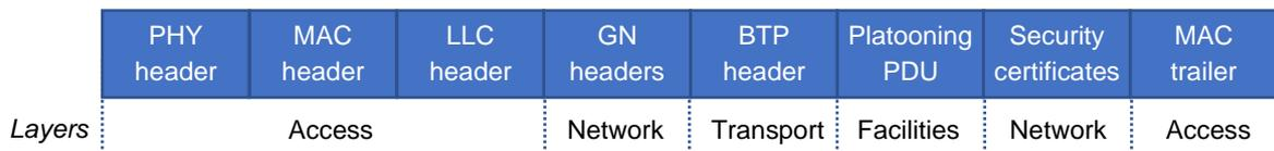
Figure 3: Packet encapsulation of the platooning PDU
