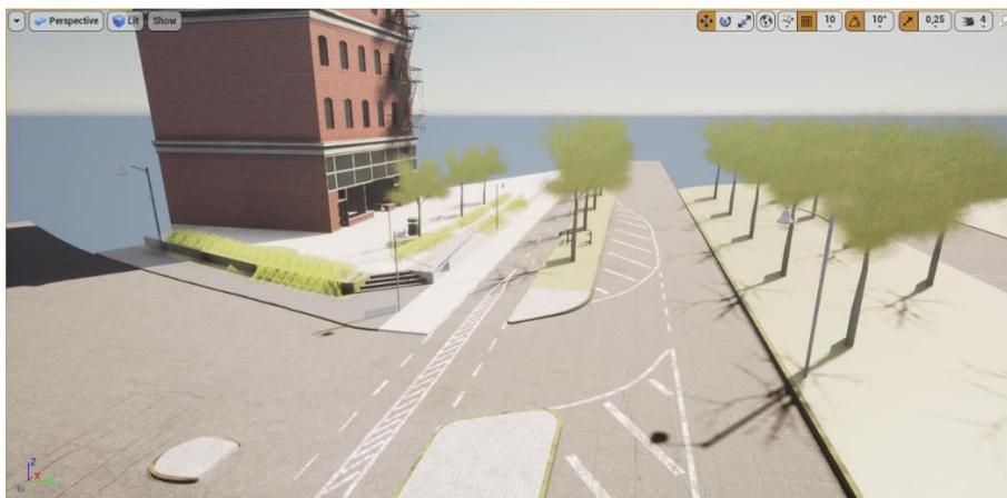
Figure 3: The digital model of the Lindholmen intersection after it was imported into CARLA. Note that some of the signs present in Figure 2 are missing. Some of the textures, particularly the leaves and the pavement material, also do not look particularly realistic.
