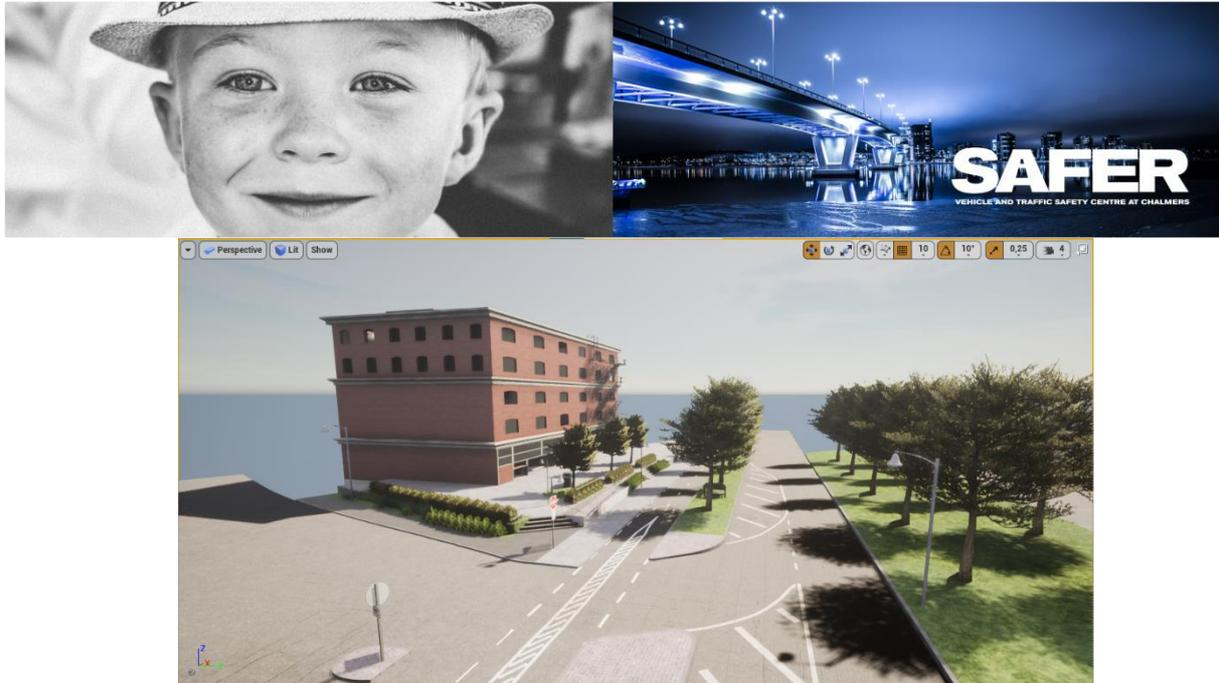
Figure 4: The improved digital model of the Lindholmen intersection after it was imported into CARLA. Compared to Figure 3, the tree and bush textures look more realistic, some ground material has been changed and some signs have been added. The building to the left in the image has also been re-scaled.
