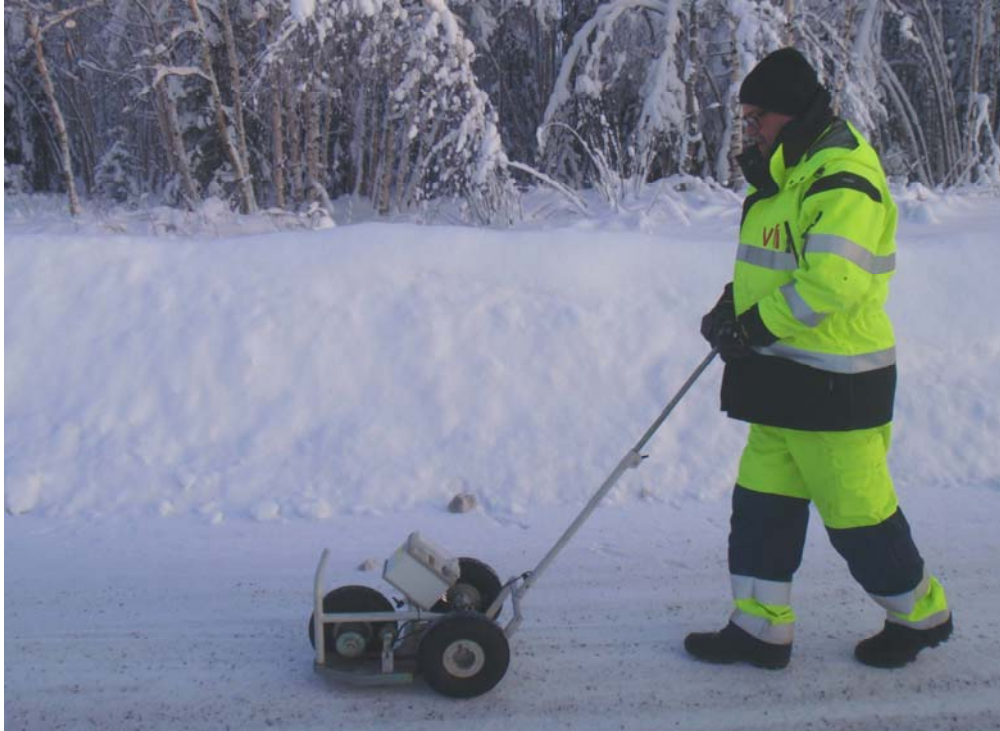
Figure 2. The Portable Friction Tester used to measure friction on cycleways.
