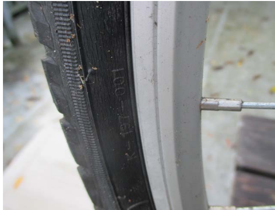
Condemning groove on aluminium rim of Asama Euro7
