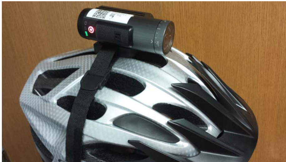
Figure 1. Pedal PORTAL data acquisition system mounted on helmet.
