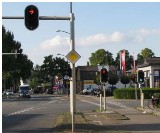
Figure 8: Example of a bike box (left) and a pre-start for cyclists, i.e. through cyclists have a green light while the light for right turning motor vehicles is still red (right)
