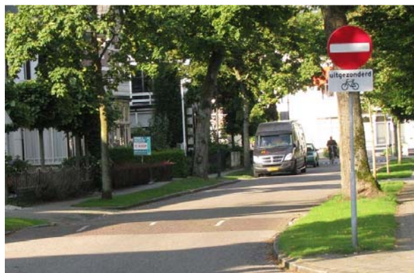
Figure 5: Example of a street closure (left) and one-way street with allowance of contraflow cycling, indicated by the traffic sign (right)
