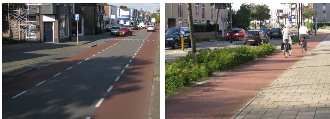
Figure 6: Example of a bicycle path (right) and bicycle lane (left)
