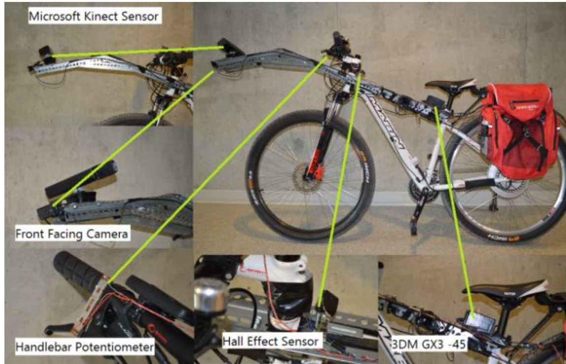
Figure 1. IPB and Mounted Sensors
