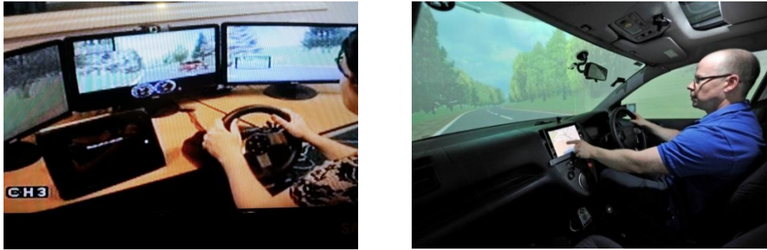
Figure 1 Low-fidelity simulator (left) and Medium fidelity simulator (right) used in this study
