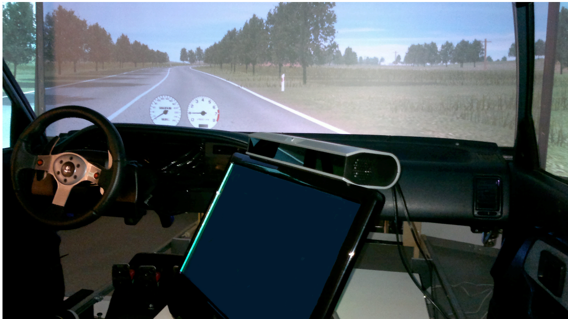
Figure 2 Inside the driving simulator with the touch monitor and remote eye tracking system. The analog HUD meters are visible above the steering wheel.
