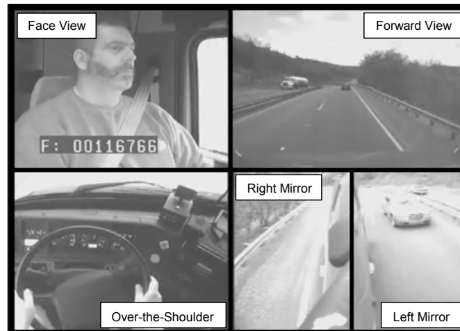
Figure 1. Split-Screen Presentation of the Five Camera Views Used in the NTDS. Driver shown is an employee of the Virginia Tech Transportation Institute.
