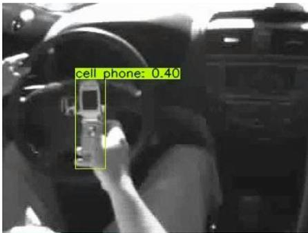
**Fig. 2.** Detected cell phone use of a driver by YOLOv4
