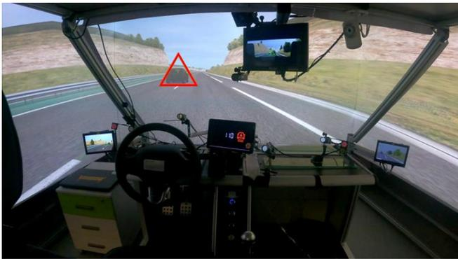
Fig. 1. Example of the situation adaptive HMI
