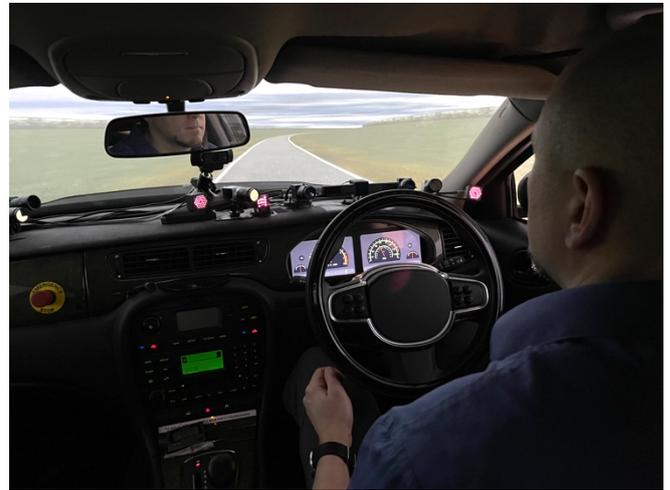
Figure 3: The setup of the experiment: occlusion drive's unoccluded period (Grahn et al. 2024b)
