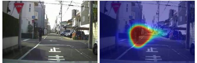
**Fig. 1.** Left: Dashcam image. Right: Driver's Focus of Attention (DFoA) as predicted when using the driver attention predictor trained with conventional dataset. While it can detect the pedestrian, it should also consider traffic signs, blind spots, etc. in this complex environment.
