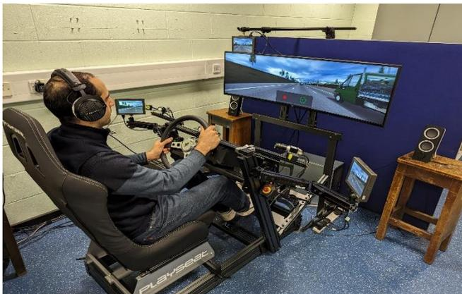
Figure 1: Static driving simulator set up.
