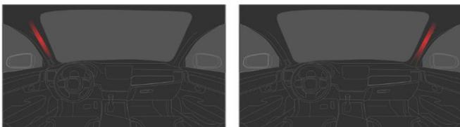
Figure 1: illustration of the location and shape of ambient light that showed the approach or breach of the lane line or lane edge.
