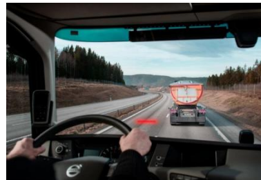
Figure 14. Volvos Distance Alert helps the driver maintain a safe distance
