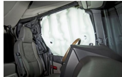
Figure 16. Side curtain airbag offered by Scania side curtain airbag is to protect the driver and passenger in case of a rollover accident.
