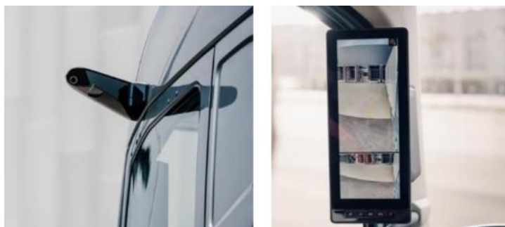
Figure 8. Digital rear view mirrors on a Volvo Truck
