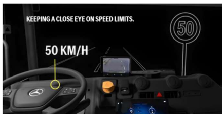
Figure 11. Speed sign information in a MB truck
