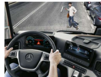
Figure 12. MB has an AEB-function that stops for vehicles and VRU.
