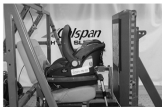
Simplified front row structure (e.g., blocker plate) [Patton et al. 2020]
