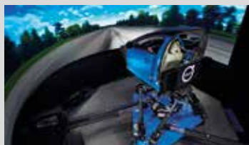
Chassis simulator, Volvo Cars
