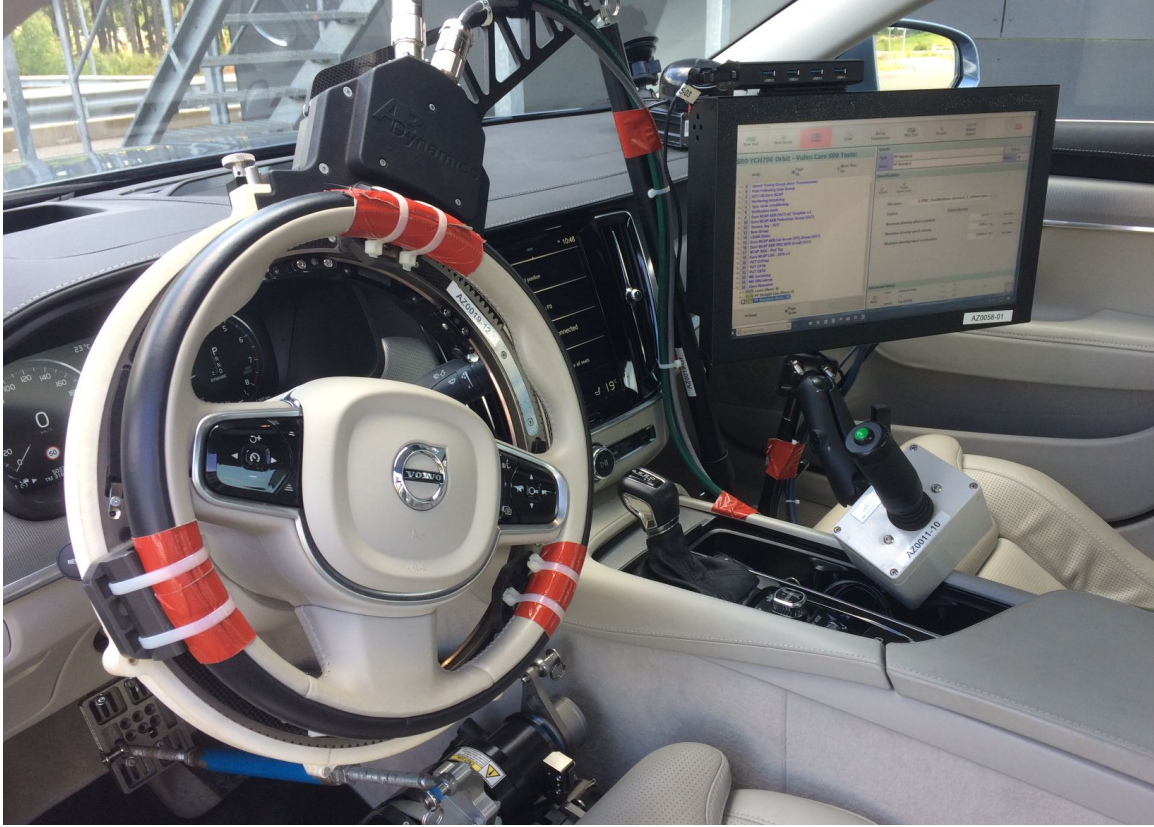
Figure 8.9: Steering robot used for executing driving trajectories.
