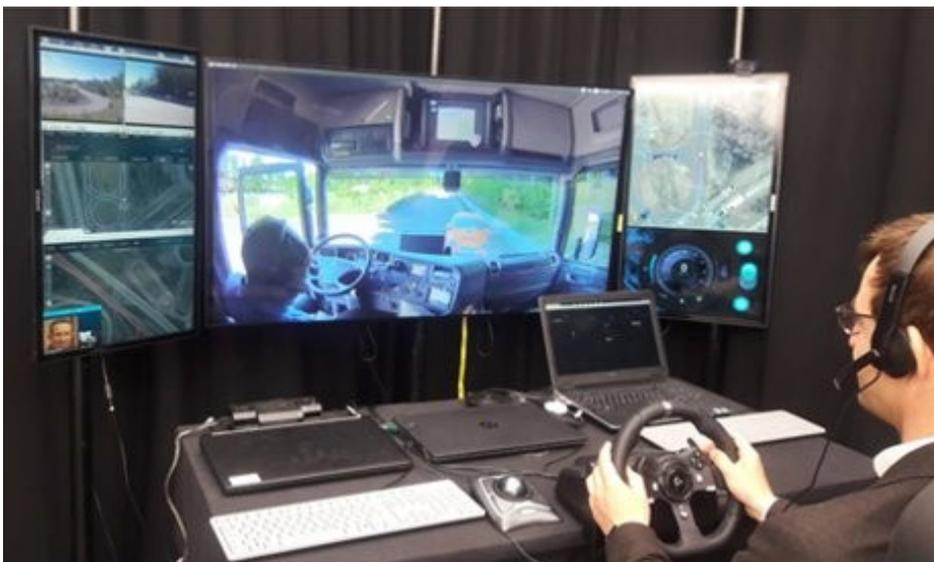
Figure 9. Remote driving station used to control the test bus during the 2017 demo.
