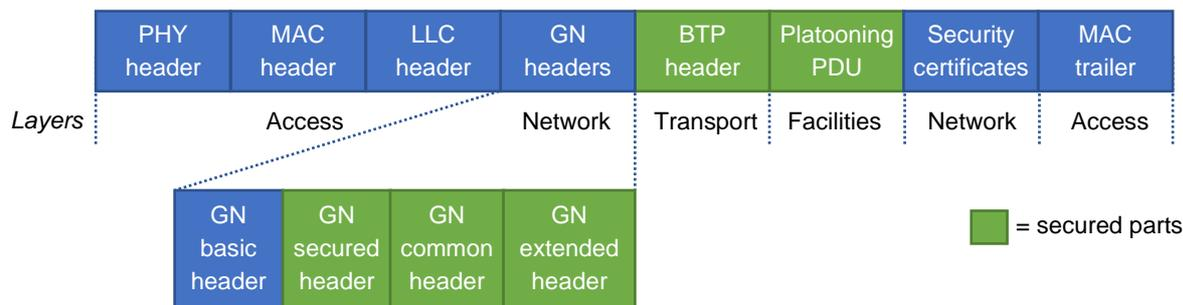
Figure 5: Secured GN encapsulation of the platooning PDU and BTP header
