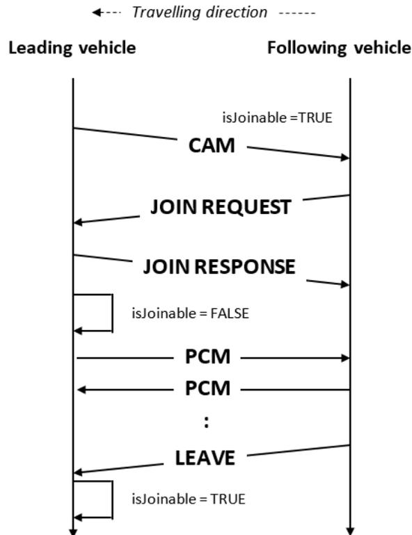
Figure 9: Overview of platooning from joining to leaving
