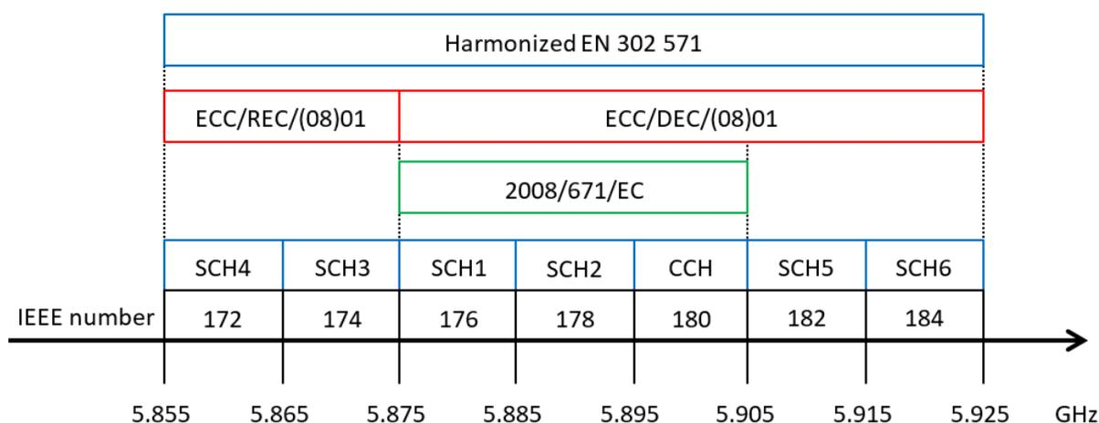
Figure 2: ITS frequency band in Europe with corresponding channel names and IEEE channel numbering
