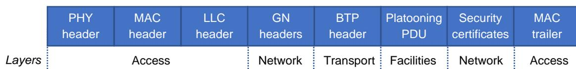
Figure 3: Packet encapsulation of the platooning PDU
