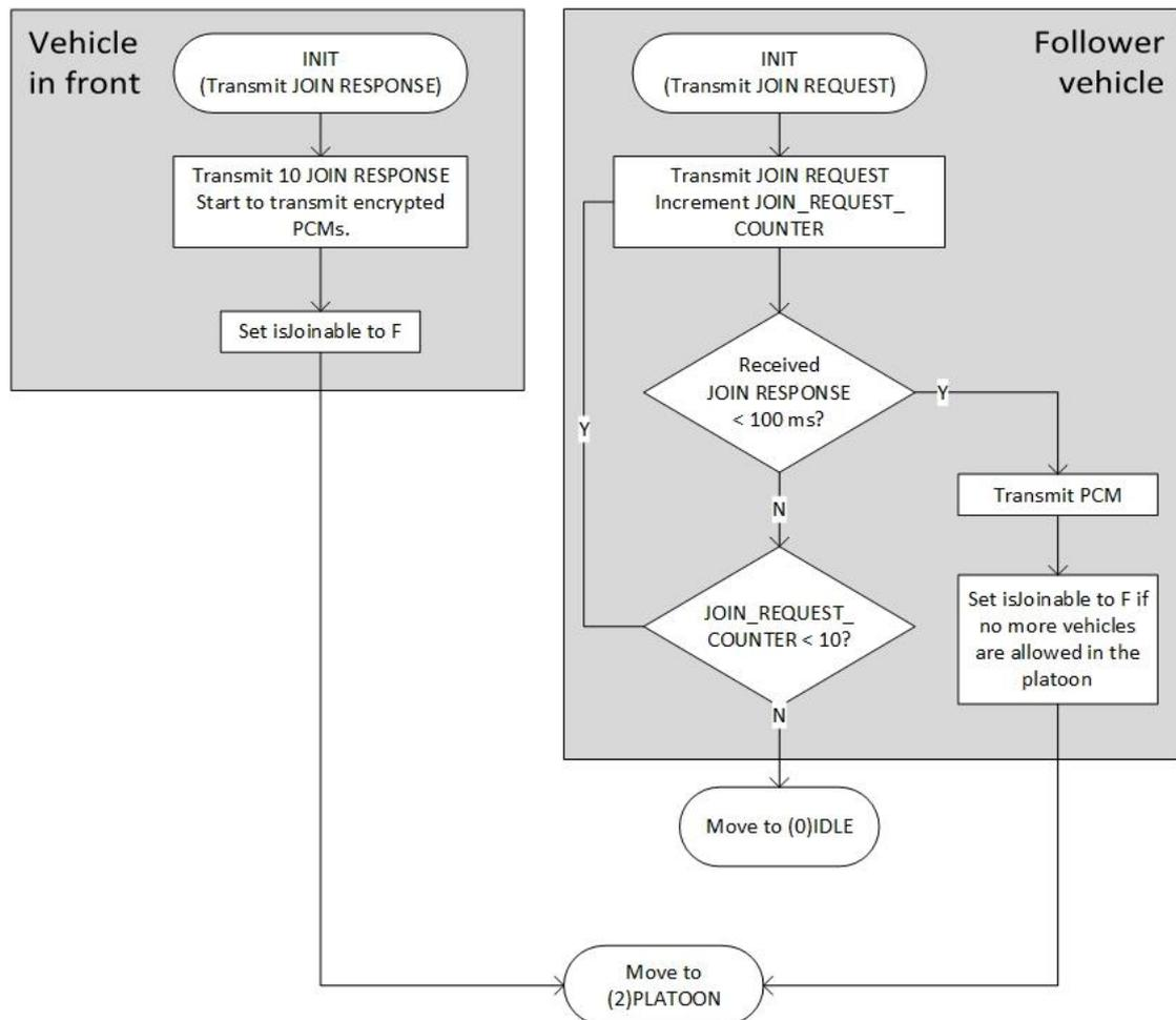
Figure 11: JOIN procedure
