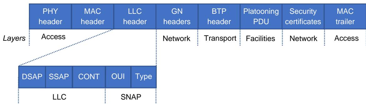
Figure 6: LLC encapsulation of the platooning PDU
