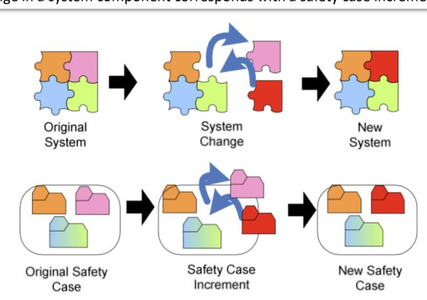
Change in a system component corresponds with a safety case increment
