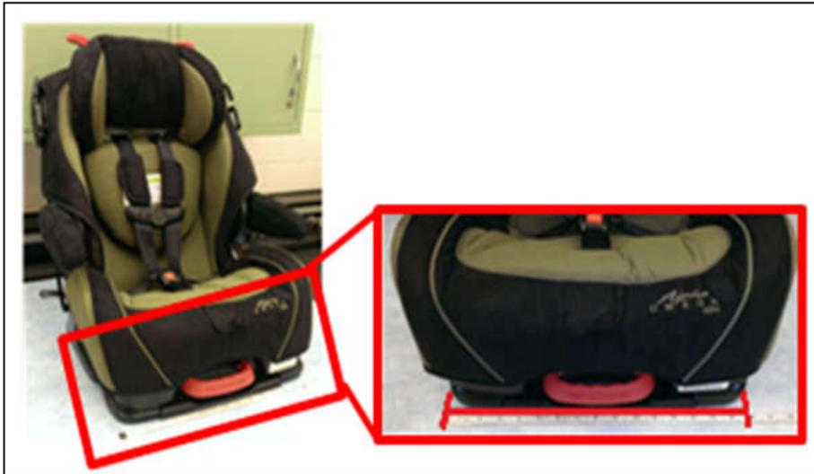
Width of edge of CRS which would be installed in the seat bight
