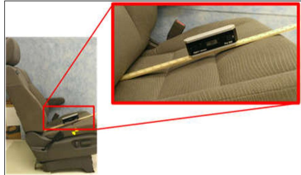
Measure seat pan angles of vehicles, using rigid stick and digital inclinometer.
