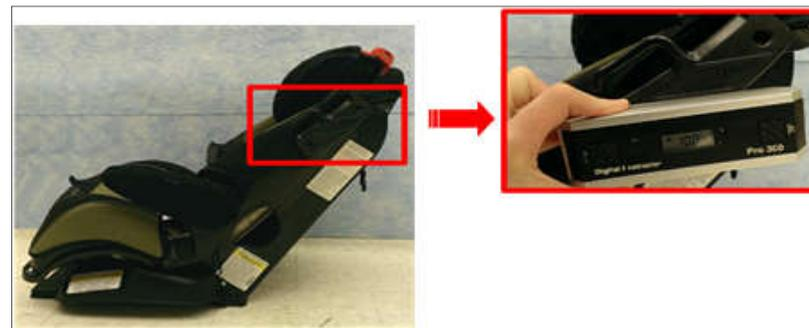
In order for their level-to-ground lines to be horizontal, both of these RF CRS must be rotated the opposite direction of any seat pan angle (clockwise as shown).
