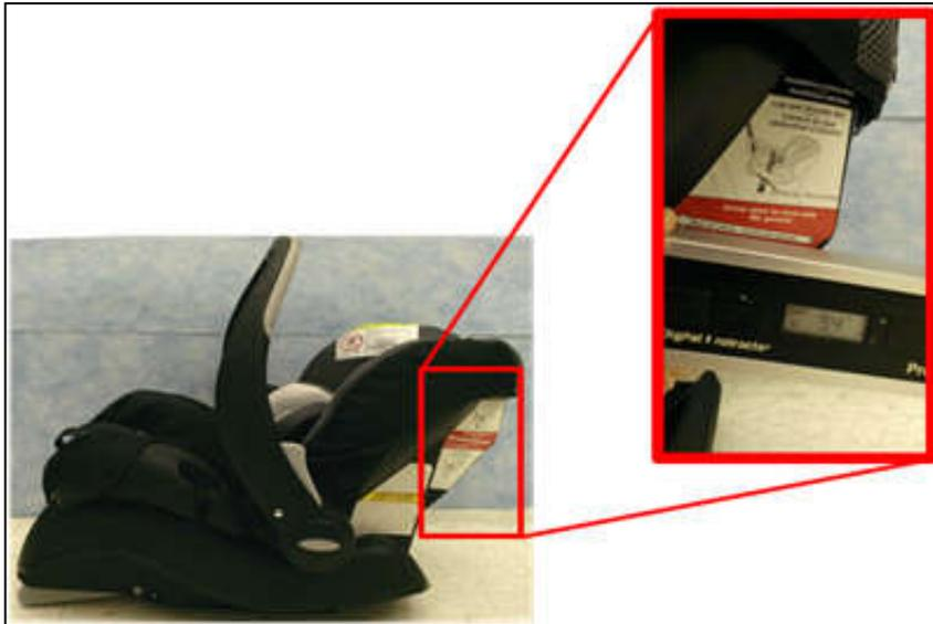
Using a digital inclinometer and the angle indicators on the side of the CRS, determine base angle range necessary for proper installation.
